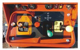
The SK650 control console uses two pilot-operated travel levers (left), a joystick-type controller for lift and tilt (green) and an auxiliary-hydraulic-system engagement lever (yellow), which is linked to a foot pedal in order to allow hands-free operation of the auxiliary system.
