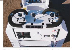
The Ramrod 1150 TD's console is designed for "palm steering" with the right hand, and auxiliary-hydraulicsystem controls allow directing either 6 or 12 gpm into the system, depending on the attachment. Steel tanks that flank the operator's station — hydraulic oil (right) and fuel (left) — swing out to allow engine access.
