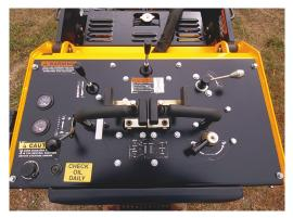
The operator controls the Boxer's steering levers, located between the handgrips, with thumbs and forefingers. Similarly controlled are the boom lever (forward of left handgrip) and bucket lever (forward of right handgrip). The auxiliary-hydraulic-circuit lever is at the upper left, and the track-width controller at top center.
