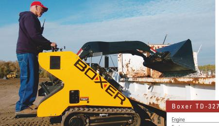
The Boxer TD-327 has a bucket-hinge-pin height of 75 inches and a dump height (at 45 degrees) of 59 inches.
