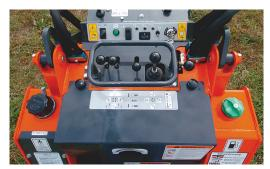
green button on the dash must be pushed to unlock all machine functions. The fuel tank (right) and hydraulic tank (left) are integral with the machine's frame.
