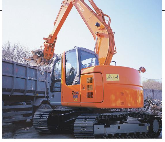
Nineteen of the 10- to 20ton excavators available today — nearly half — are reduced-swing-radius, or zero-swing-radius machines like Hitachi's Zaxis. Recent innovation in this class of excavators has been dominated by introduction of reduced-radius machines.
