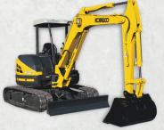
short radius. Four highly-maneuverable models designed to work in crowded spaces. Operating weights from 31,750 to 57,300 lbs. 84 to 148 HP.
